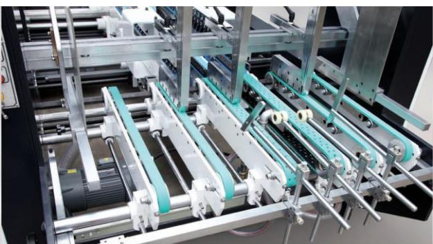
auto feed correctly and continuously, internal of feeding is adjusted by continuously variable speeder; independent high-speed feeding bell can be easily adjusted; independent vibrating motor can improve feeding greatly; feeding blade and baffle on the left and right can be adjusted upper and down to shorten adjusting and carton changing time.
